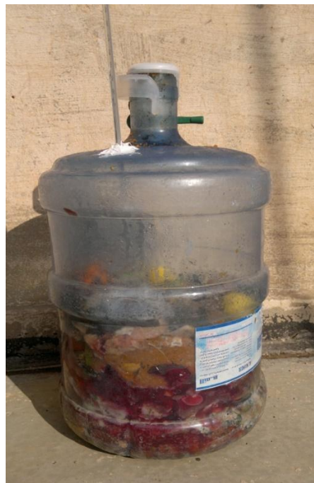
Figure 2: The in-vessel composting reactor with raw materials.
